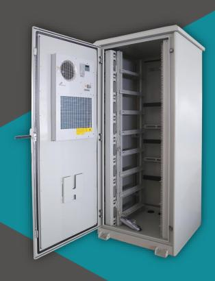
Between the inside and outside side panel has the inter space, which provides the channel to ventilate and support the enclosure internal heat exchange, and also can reduce the influence of the sunlight illumination.
